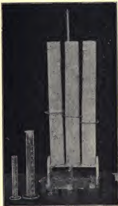
FIG. 58. Movement of Water through Soils.
